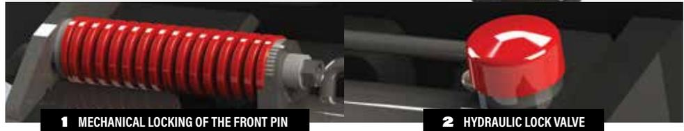
1 MECHANICAL LOCKING OF THE FRONT PIN
